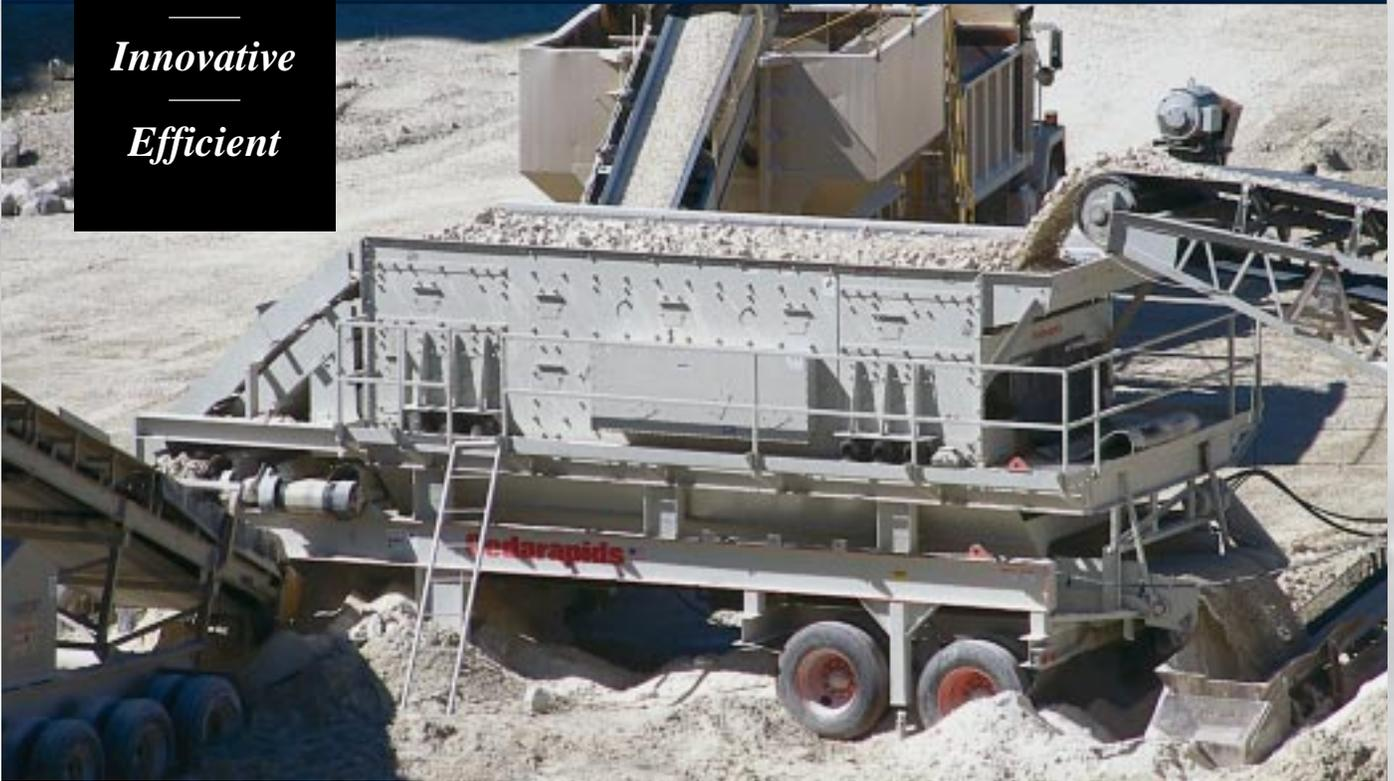
*Cedarapids/ElJay Legacy Series Screens provide the contractor with proven performance. The ability to change stroke angle, amplitude and speed to meet changing screening conditions makes this versatile screen highly efficient in most any application. Smooth operation, virtually non-plugging, exceptional bearing life and simplified adjustment procedure make the Legacy ideal for either stationary or portable applications.*
